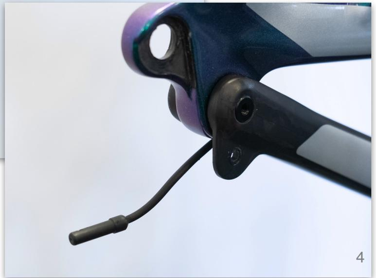
4. Separate the sensor from the bracket.
