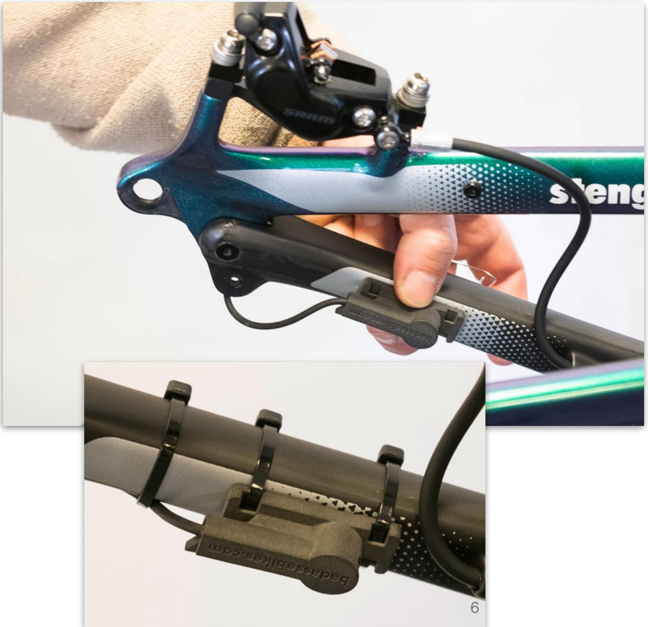
6. Attach the adapter and the cable of the sensor to the frame of your bike with cable ties.
