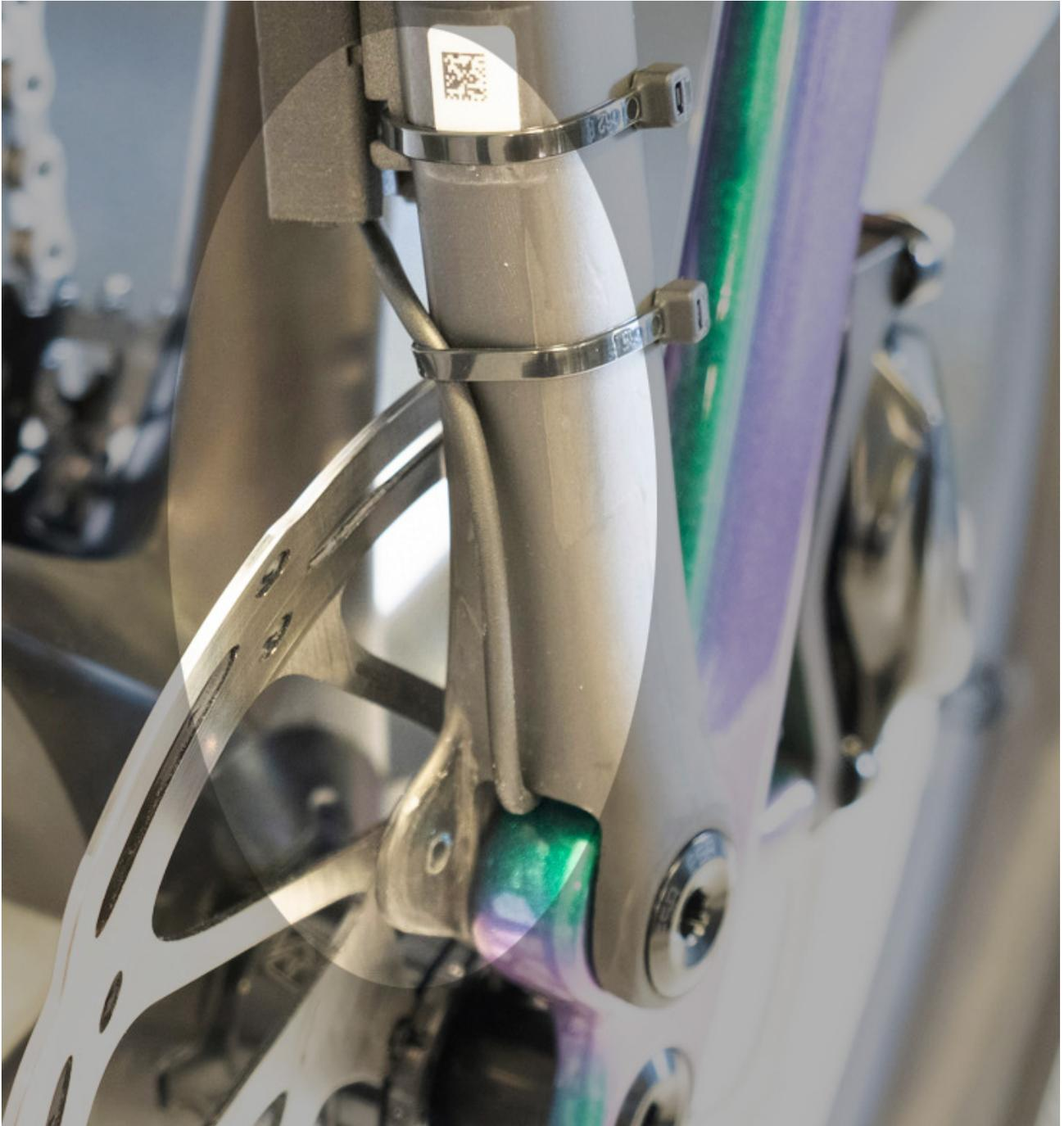
**Attention** Make sure that the cable of the sensor is securely fastened and that it cannot reach the brake disc under any circumstances.
