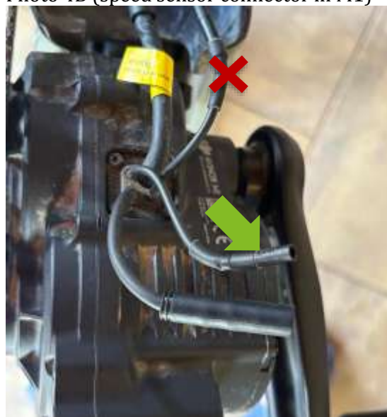
Photo 4B (speed sensor connector in M1)
