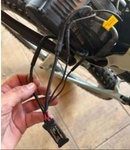
Photo 5A (connected chip in M1 motor)
