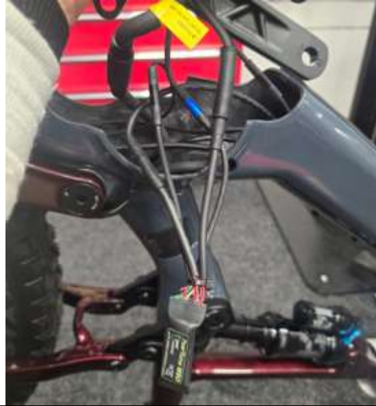
Photo 5B (connected chip in M2 motor)
