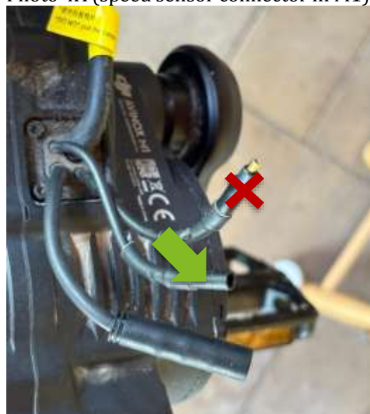
Photo 4A (speed sensor connector in M1)
