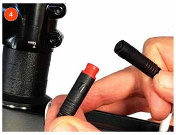
Disconnect the connector with the middle red line.
