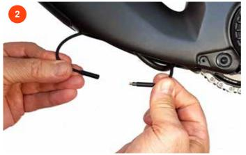
Disconnect the connector. DO NOT PULL BY THE CABLES but by the rigid plastic part.
