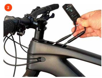
Extract the display by removing the central screw that fixes it to the frame.
