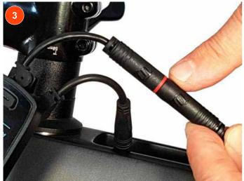
Locate the connector with the middle red line.
