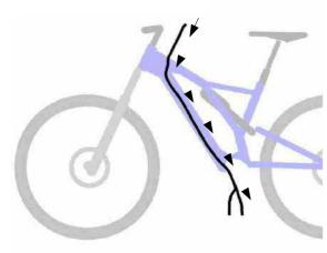
Insert connectors 3 and 4 from the hole in which the display was housed and reach the engine passing inside the diagonal tube of the frame (battery housing). We suggest using a "wire puller". Only if necessary remove the battery.
