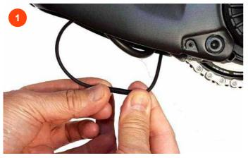
Locate the connector that connects the speed sensor to the motor.
